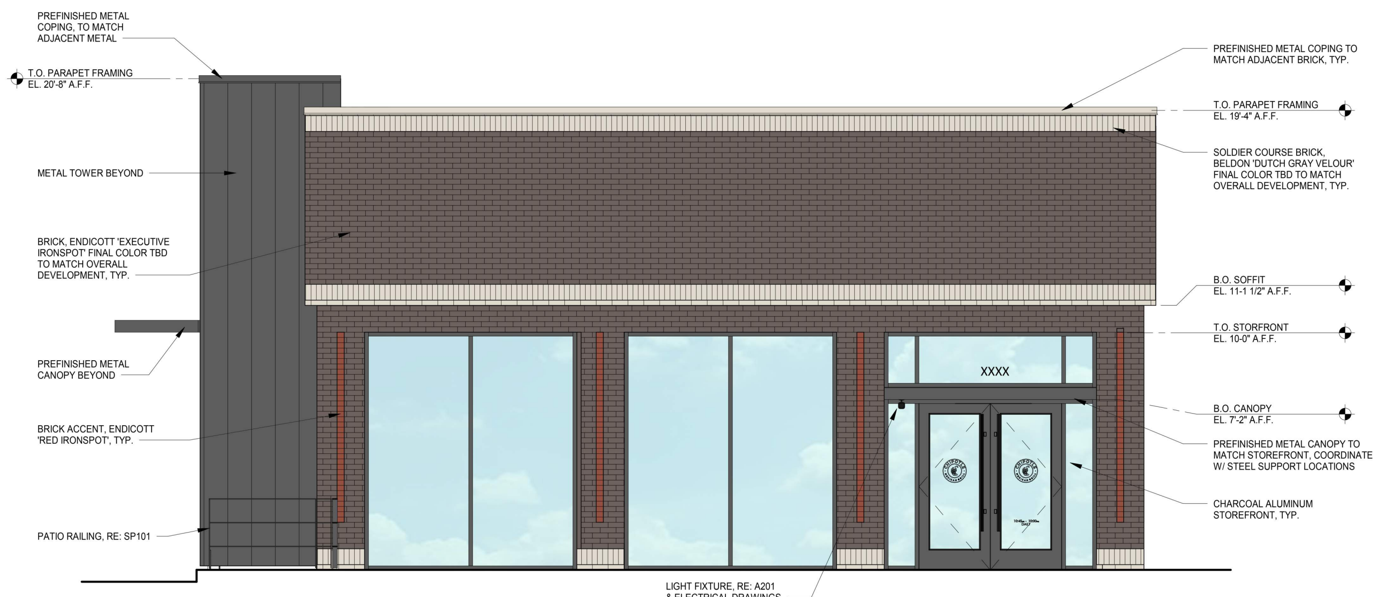
2 EXTERIOR ELEVATION - SOUTH 1/4" = 1'-0"
