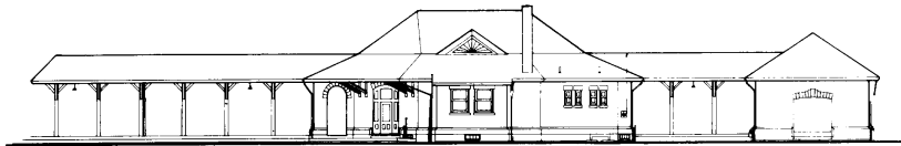
404 Railroad Station. Williamstown, Massachusetts. 1898. Representative of a type built during the peak years of rail modernization, electrification, and consolidation. Characteristic are the double-pitched roof and its canopy extensions.
